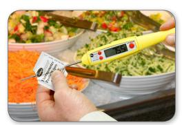
If there is no display when the thermometer is turned on, check the condition of the batteries. Also check that the battery terminals are clean and batteries are properly installed. If batteries show signs of corrosion, remove immediately and replace. Refer to the product Operating Instructions or User Guide and Instrument Warranty booklet for battery installation and replacement guidelines. Always wash, rinse and sanitize these products.
