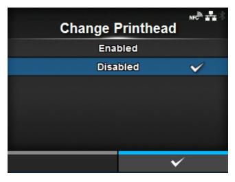
Enable or disable the notification function about when the print head needs to be replaced.
