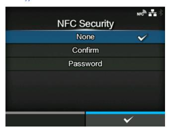
Set whether to show the confirmation message or enable the password input before settings are written to the product from an Android device with the NFC interface.
