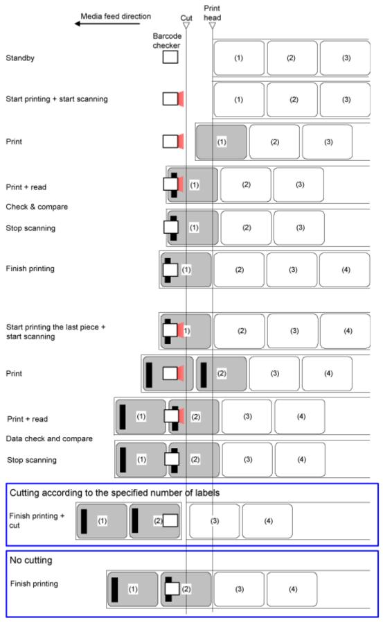
Operation 53: Cut & Print Mode When the Barcode Check Function Is Enabled
