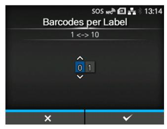
Specify the number of barcodes per label when you include barcodes which are not created by barcode commands as the target of the barcode readability check.
