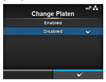
Enable or disable the notification function about when the platen roller needs to be replaced.
