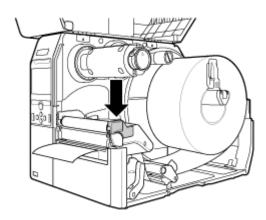
8. Press the media guide (4) lightly against the end of the media, and turn the knob (5) to lock the media guide.
