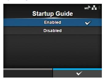
The startup guide is a function to help you through the initial product settings (such as setting date and time, and loading the ribbon and media).
