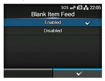
Set whether to feed a label with nothing printed on it when the product receives label formatting commands that do not generate any printable image.
