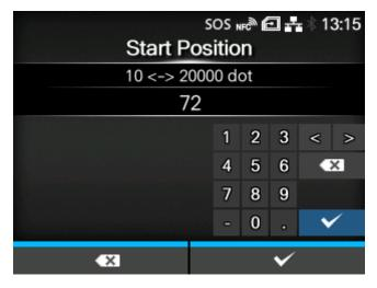
Adjust the position at which the barcode check starts (position of the barcode checker at which reading starts).
