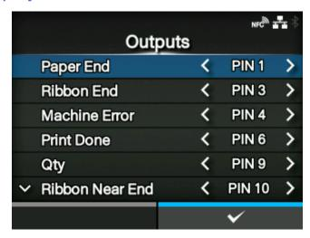
Assign the pin No. to output signals.
