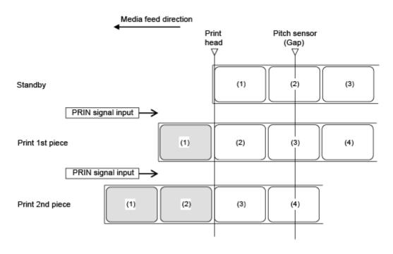
The figure above shows the reference position when the Gap sensor is used.
