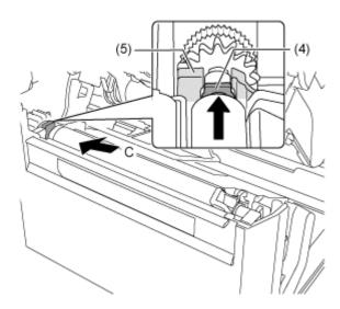
b. Next, make sure that the tab (6) on the right driven end of the platen roller is pointing upward. Push the platen roller again in the direction C so that the tab (6) is fixed in the groove (7) at the driven side.
