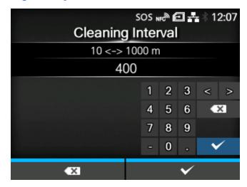
Set the notification interval about when the print head needs to be cleaned.
