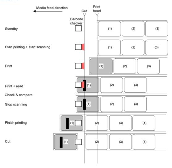
Operation 52: Cutter Mode (Cutting According to the Specified Number of Labels, No Cutting) When the Barcode Check Function Is Enabled
