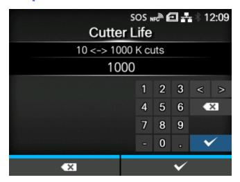
Set the notification interval about when the cutter unit needs to be replaced.
