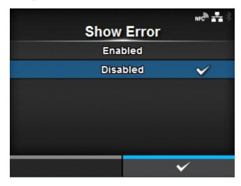
Enable or disable the command error indication when incorrect command or parameter is detected in the print data.
