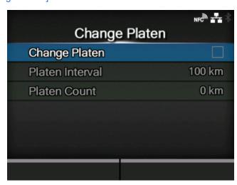
Notify when the platen roller needs to be replaced.
