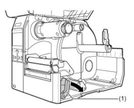
4. Lift the lever (2) in the direction A to unlock the platen roller (3), and then pull out the platen roller (3) in the direction B.
