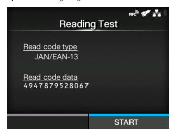
If the reading is unsuccessful, or if the displayed read result is not correct, adjust the position of the barcode checker by operating the barcode checker stand. For details on how to use the barcode checker stand, refer to the Barcode Checker Stand Kit Installation Manual that came with the barcode checker stand kit.
