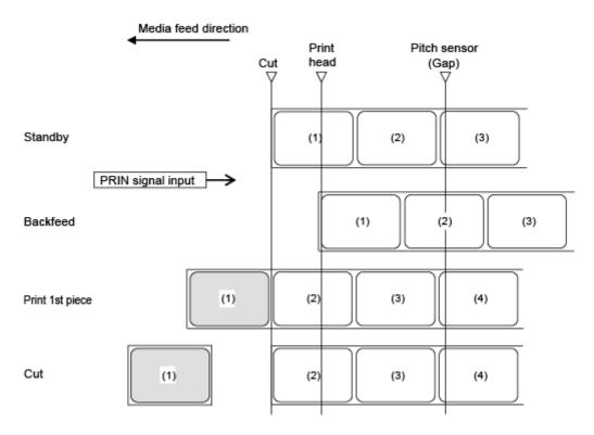
The figure above shows the reference position when the Gap sensor is used.
