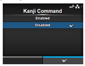
Set the product behavior when the received data includes the Kanji command ESC+K5, ESC+K6 or ESC+K7.
