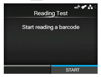
If reading is successful, the barcode type and data read are displayed on the screen. Only the first 23 bytes of data are displayed.
