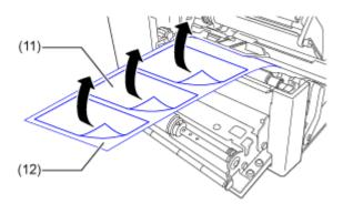
9. Pass the liner (12) through the gap of the dispenser unit to the outside of the product.
