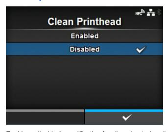
Enable or disable the notification function about when the print head needs to be cleaned.
