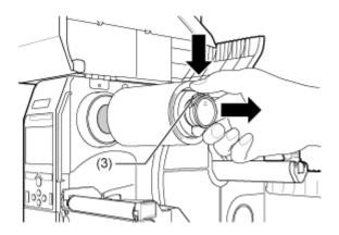
4. Pull to remove the used ribbon from the ribbon rewind spindle.
