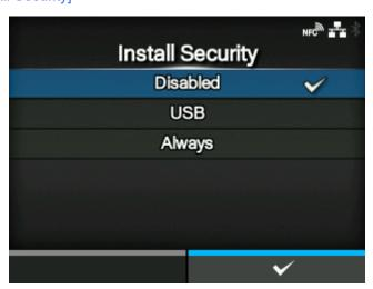
Enable or disable the password input for installing the pkg file to the product.
