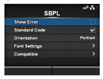
SBPL (SATO Barcode Printer Language) is the common command that controls SATO barcode label printers.
