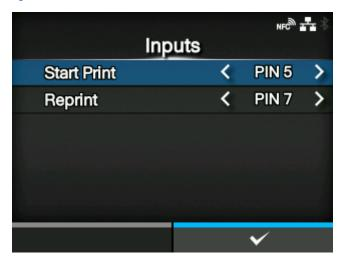
Assign the pin No. to the input signals Print Start and Reprint.
