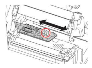
• The I-mark sensor (reflective type) is below the ☐ mark, and the Gap sensor (transmissive type) is below the ▽ mark.
