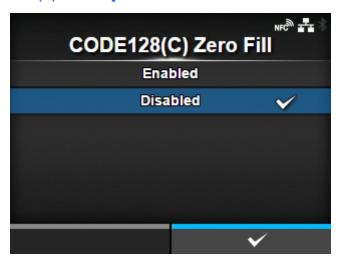
Set whether to allow odd digits and print the barcode with zero-filling at the end of the data when start code C is used in CODE128.
