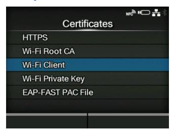
Install certificates used for Wi-Fi authentication and for HTTPS.
