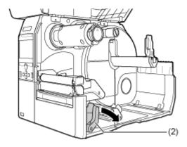
3. Place the fan-fold media on a flat location, and load the media from the media slot on the rear or the bottom of the product.
