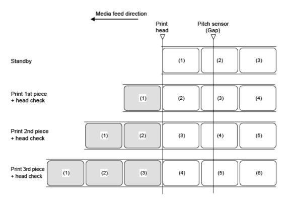
The figure above shows the reference position when the Gap sensor is used.
