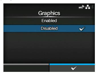
Set whether to allow the registration of graphic data even if a line feed code is omitted.
