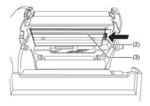
6. Disconnect all the connectors (4) from the defective print head (3).
