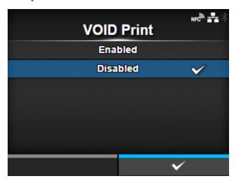
Set whether to print error marks on the media when a barcode reading error or barcode comparison error occurs.
