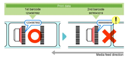
A reading error occurs if the number of barcodes in the print data is not read within the printing
