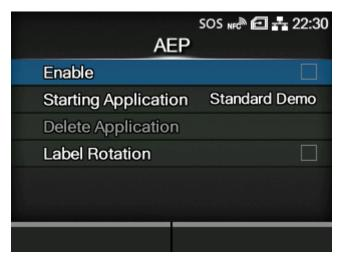
Set the functions for AEP (Application Enabled Printing).
