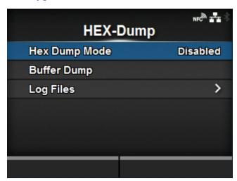
Save the hex dump print data or dump data from the receive buffer to the USB memory.
