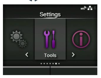
5. Press the ▲/▼ buttons to select [Barcode Checker] > [Test] > [Interface], and then press the ← button.
