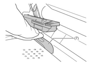
9. Return the media sensor guide to its original position and tilt the sensor guide lock up to the locked position.
