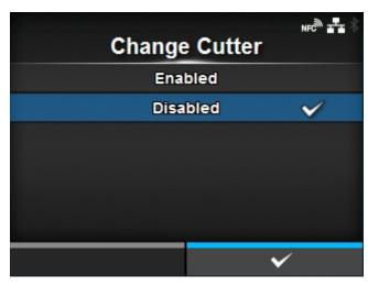
Enable or disable the notification function about when the cutter unit needs to be replaced.
