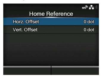
Adjust the print reference position by specifying the offset position in the horizontal and vertical directions.
