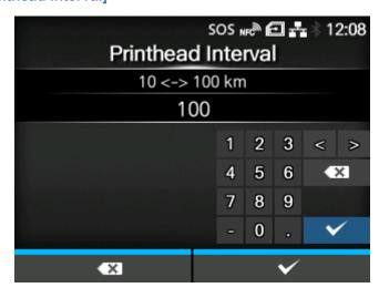
Set the notification interval about when the print head needs to be replaced.
