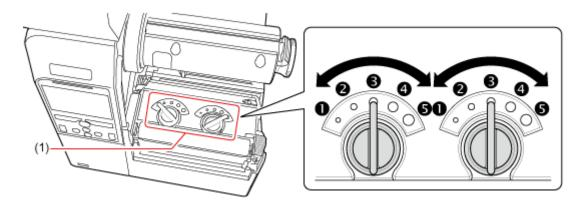
3. Turn the adjustment dials (1) according to the media width and set the pressure balance.
