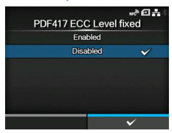
Set whether to print the PDF417 code with the security level specified by the PDF417 printing command.
