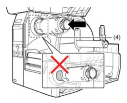
6. Remove the used ribbon core from the ribbon supply spindle.
