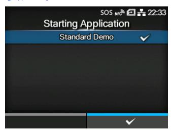
Select the application to start at product startup in AEP (Application Enabled Printing) mode.
