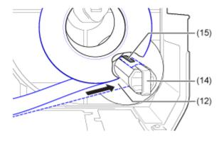
12. Rotate the liner rewinder (14) counterclockwise by hand, to wind the liner.
