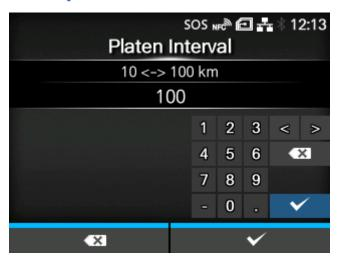
Set the notification interval about when the platen roller needs to be replaced.
