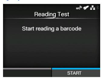
Perform a test read with the connected barcode checker.
