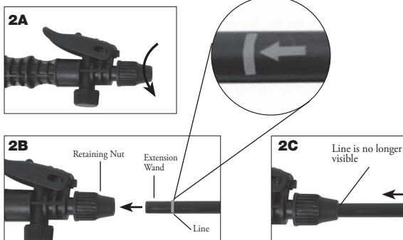
Loosen retaining nut from shut-off (2A). Insert extension wand into end of shut-off until you no longer see the line marked on the end of the wand. Tighten retaining nut (2C).
