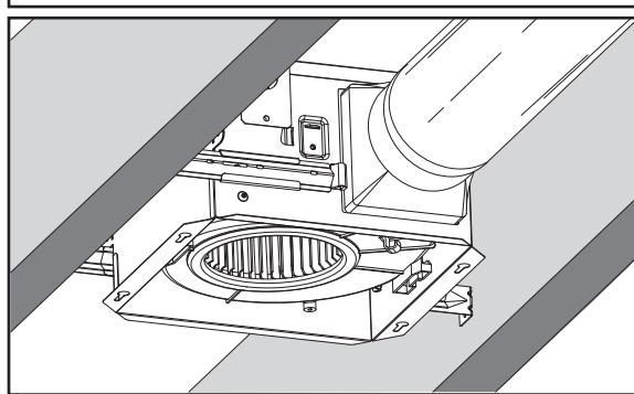
The ducting from this fan to the outside of building has a strong effect on the air flow, noise and energy use of the fan. Use the shortest, straightest duct routing possible for best performance, and avoid installing the fan with smaller ducts than recommended. Insulation around the ducts can reduce energy loss and inhibit mold growth. Fans installed with existing ducts may not achieve their rated air flow.
