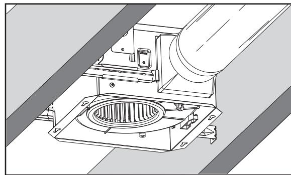
The ducting from this fan to the outside of building has a strong effect on the air flow, noise and energy use of the fan. Use the shortest, straightest duct routing possible for best performance, and avoid installing the fan with smaller ducts than recommended. Insulation around the ducts can reduce energy loss and inhibit mold growth. Fans installed with existing ducts may not achieve their rated air flow.
