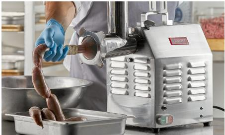
Choosing the correct sized stuffer tube in relation to the casing and type of sausage is vital to making the stuffing process much easier. Use the charts below to determine which stuffer tube to use with your Avantco Meat Grinder.
