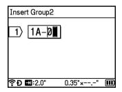
5 For the second serialized text, select [Type], [Format], [From], [To] and [Increased by] using the ↑ or ↓ key, set the values using the ← or → key, and then press the OK or Enter key.
