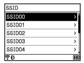
7 Select the SSID using the ↑ or ↓ key, or select [Other...] and enter the SSID (from 1 to 32 characters), and then press the **OK** or **Enter** key.
