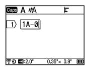
2 Position the cursor where you want to insert the first serialized text (to the right of "0"), and then press the **Shift** and **Serialize/Adv. Serialize** keys. Select [Group] using the ↑ or ↓ key, and then press the **OK** or **Enter** key.
