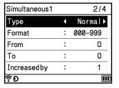
3 For the first serialized text, select [Type], [Format], [From], [To] and [Increased by] using the ↑ or ↓ key, set the values using the ← or → key, and then press the OK or Enter key.
