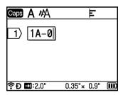
Position the cursor where you want to insert the first serialized text (to the right of "0"), and then press the Shift and Serialize/Adv. Serialize keys. Select [Simultaneous] using the ↑ or ↓ key, and then press the OK or Enter key.
