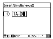
5 For the second serialized text, select [Type], [Format], [From], and [Increased by] using the ↑ or ↓ key, set the values using the ← or → key, and then press the **OK** or **Enter** key.
