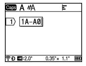
Position the cursor where you want to insert serialized text, and then press the Serialize/Adv. Serialize key.
