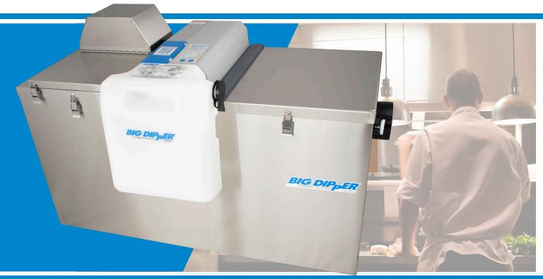
The Big Dipper automatic grease removal device lets you take control of grease and small food particles in an easier and more hygienic way. Its electrical assembly includes a heater, skimming wheel and skim setting controls that work together to remove grease from the tank and store it in a separate grease collector.
