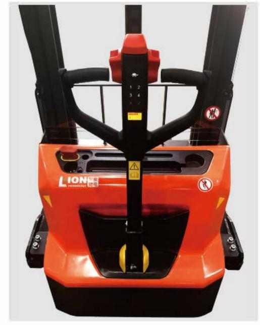
The operator can always clearly see the forks which significantly increases safety of operation.
