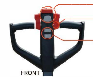
Emergency-reverse & Horn Buttons Dual butterfly-style thumb driving controls
