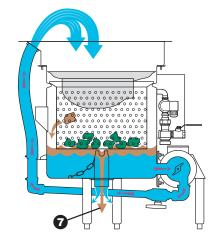
**7** Excess waste water flows into the drain.
