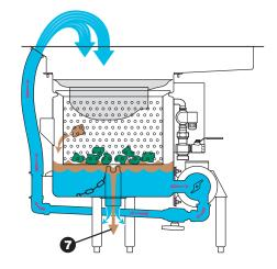
**?** Excess waste water flows into the drain.
