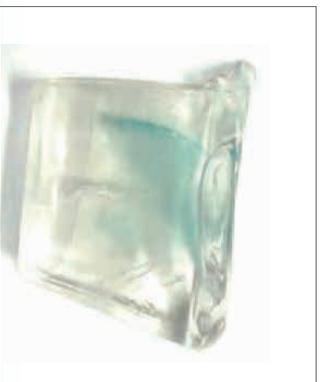
Turbulent water over the grid cell design traps air and impurities causing soft, cloudy ice that melts faster. *Blue represents impurities trapped in ice.*
