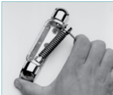
2. Place thrust washer and bushing over hexagon pin on mounted hinge. Insert adjustment pin into adjustment bushing assembly. Grasping adjustment pin, compress spring and place adjustment bushing assembly over round pin.
