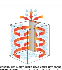
**CONTROLLED MOISTURIZED HEAT REEPS HOT FOODS FRESH LONGER** Hatco's Flav-R-Savor® air flow pattern is designed to maintain consistent cabinet temperature without drying out foods. The precise combination of heat and humidity creates a "blanket" effect around the food. The air flow rate enables the cabinet to recover temperature rapidly after opening and closing the door.
