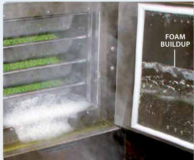
Typical connectionless steamer performance without drain.
