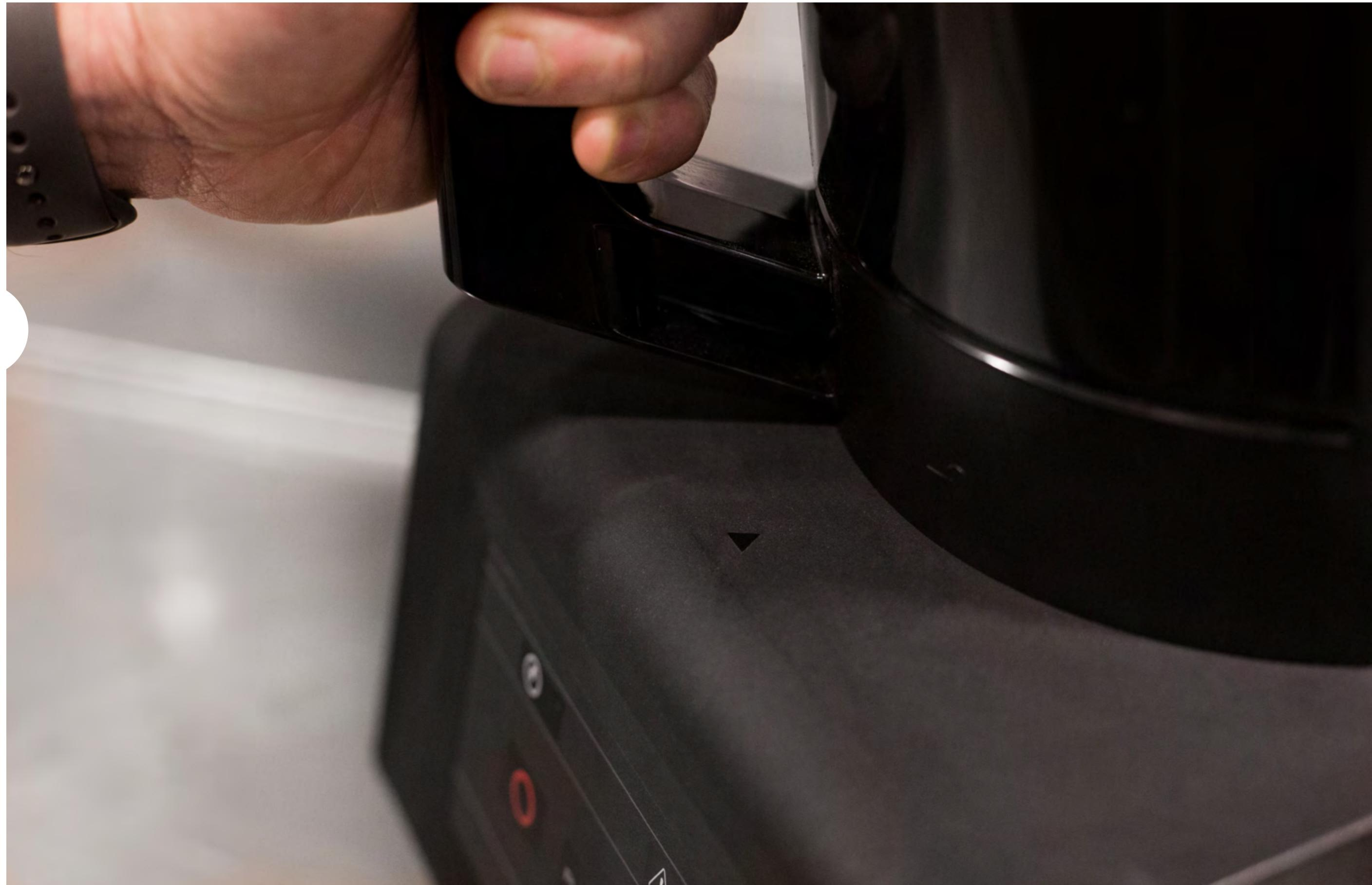
All cutters and emulsifiers K/KE have combination of safety systems that ensure user protection when the machine is in operation. The position of the bowl and its cover have microswitches that prevent them from being inadvertently switched on and the shut-off safety element prevents accidental start-up of the blades in case of power failure.
