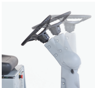
Steering is adjustable to five positions for operator comfort.
