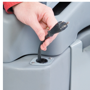
Easy access to optional onboard-charger plug.
