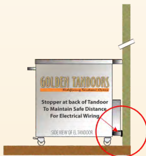
BACK STOPPERS STAINLESS STEEL WITH RUBBER MOUNTS FOR MAINTAINING DISTANCE FROM WALL TO THE EQUIPMENT Square Models Only
