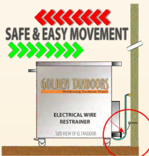
WIRE HOSE RESTRAINER TO ENSURE THE HOSE IS NEVER PULLED WHEN MOVING TANDOOR FOR CLEANING IN THE KITCHEN Square Models Only
