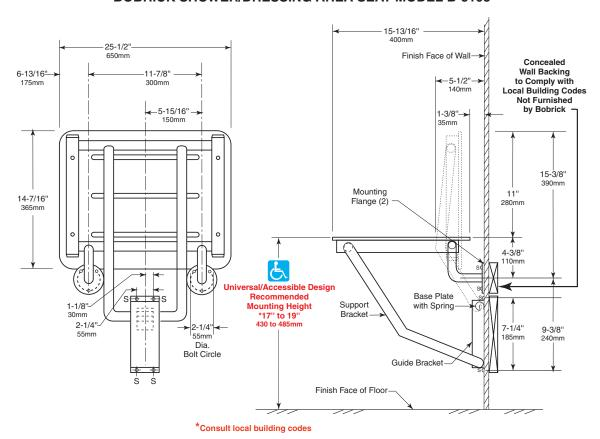
**Installation to Wall.** Secure unit to wall at points indicated by an *S*, with the two Mounting Flanges located at top and the Baseplate and Guide Bracket below. The bottom of the Support Tube must be positioned within the Baseplate and Guide Bracket before they are secured to wall. \* Mounting height of shower seat must comply with local building codes.
