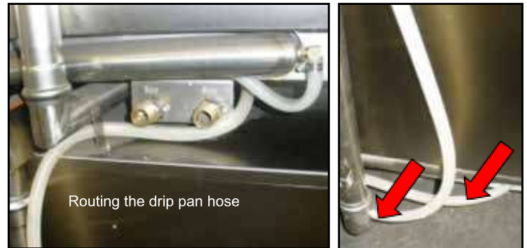
Connecting the hose to the nipple on the drain
