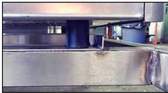
Bottom oven sitting flat, front feet behind welded stops
