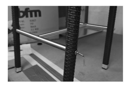
3. Wrench tighten the 4 bolts and washers as shown.
