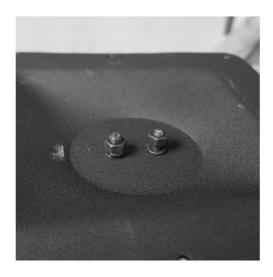
2. To attach the base plate, insert bolt with washer and tighten with wrench.
