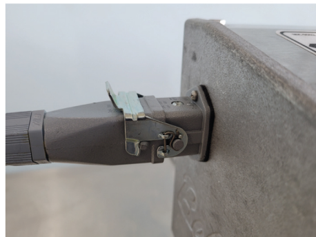
30 Plug cutter head into fryer
