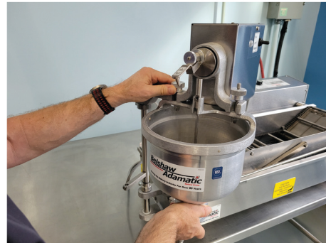
25 Install hopper onto cutter head
