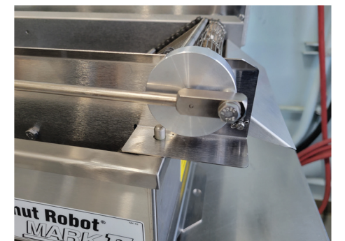
41 Stop conveyor with connecting rod to right
