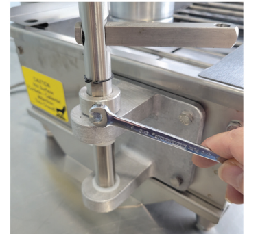
29 Loosen set screw adjust with 5/16 wrench
