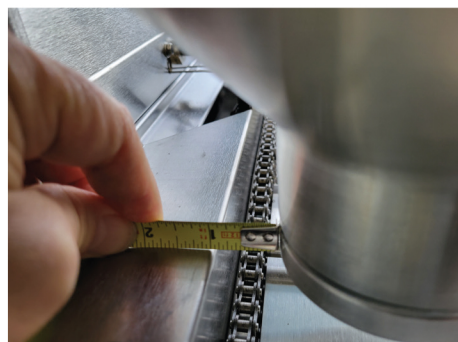
42 Check hopper is 1 inch from side panel
