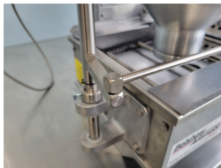
38 Attach connecting rod to swing arm
