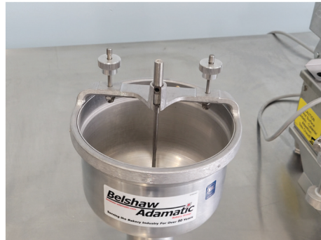
24 Install plunger into hopper
