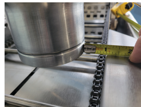
39 Adjust hopper 1 inch from side panel
