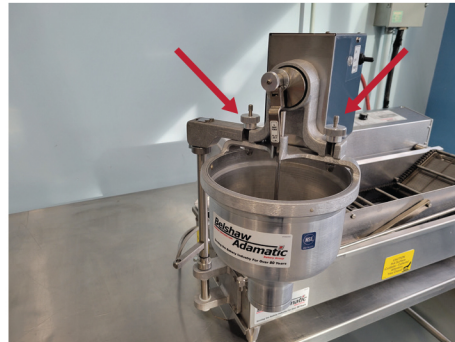
26 Tighten hopper mounting nuts
