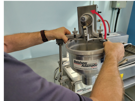
27 Lift and swing hopper over conveyor
