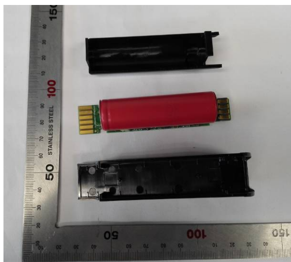
保护板/protective circuit
