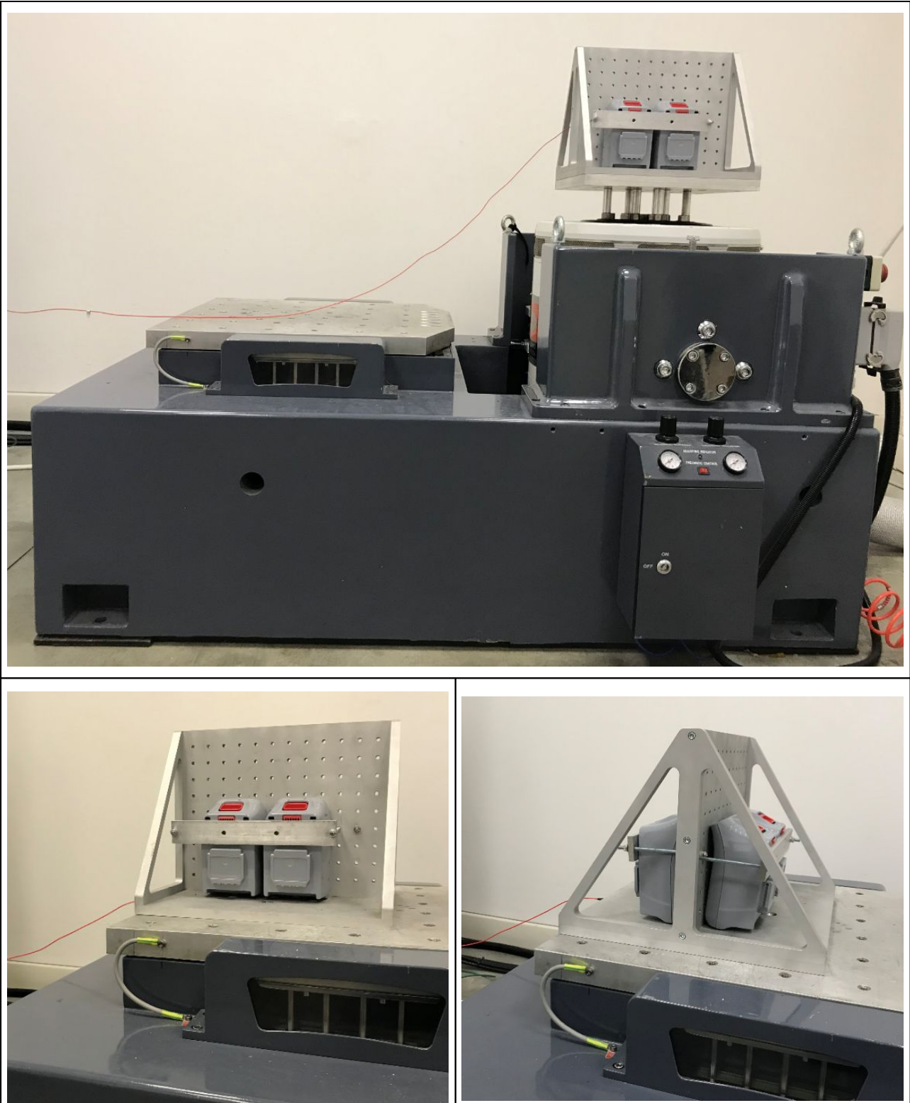
Fig. 2.5 Batteries in T.3/T.4 Test setup (Vibration/Shock test)
