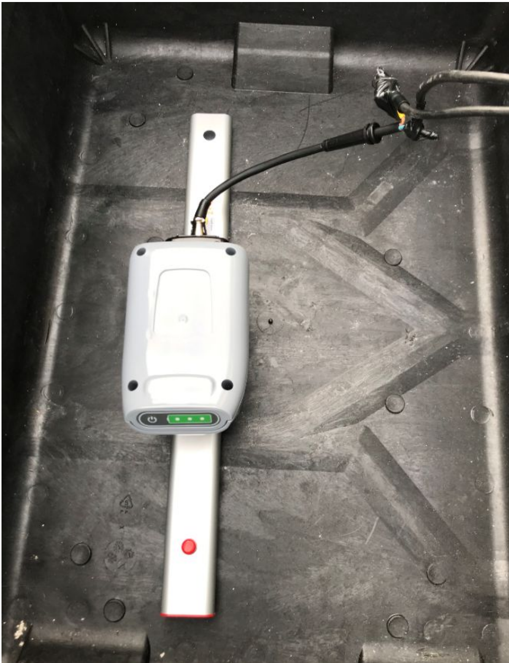
Fig. 2.6 Battery in T.5 Test setup (External short circuits)
