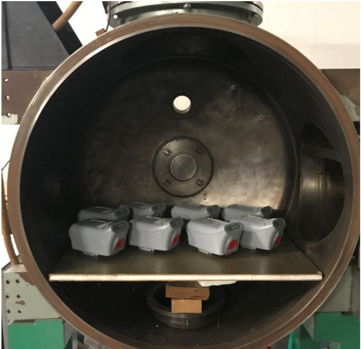
Fig. 2.3 Batteries in T.1 Test setup (Altitude Simulation test)
