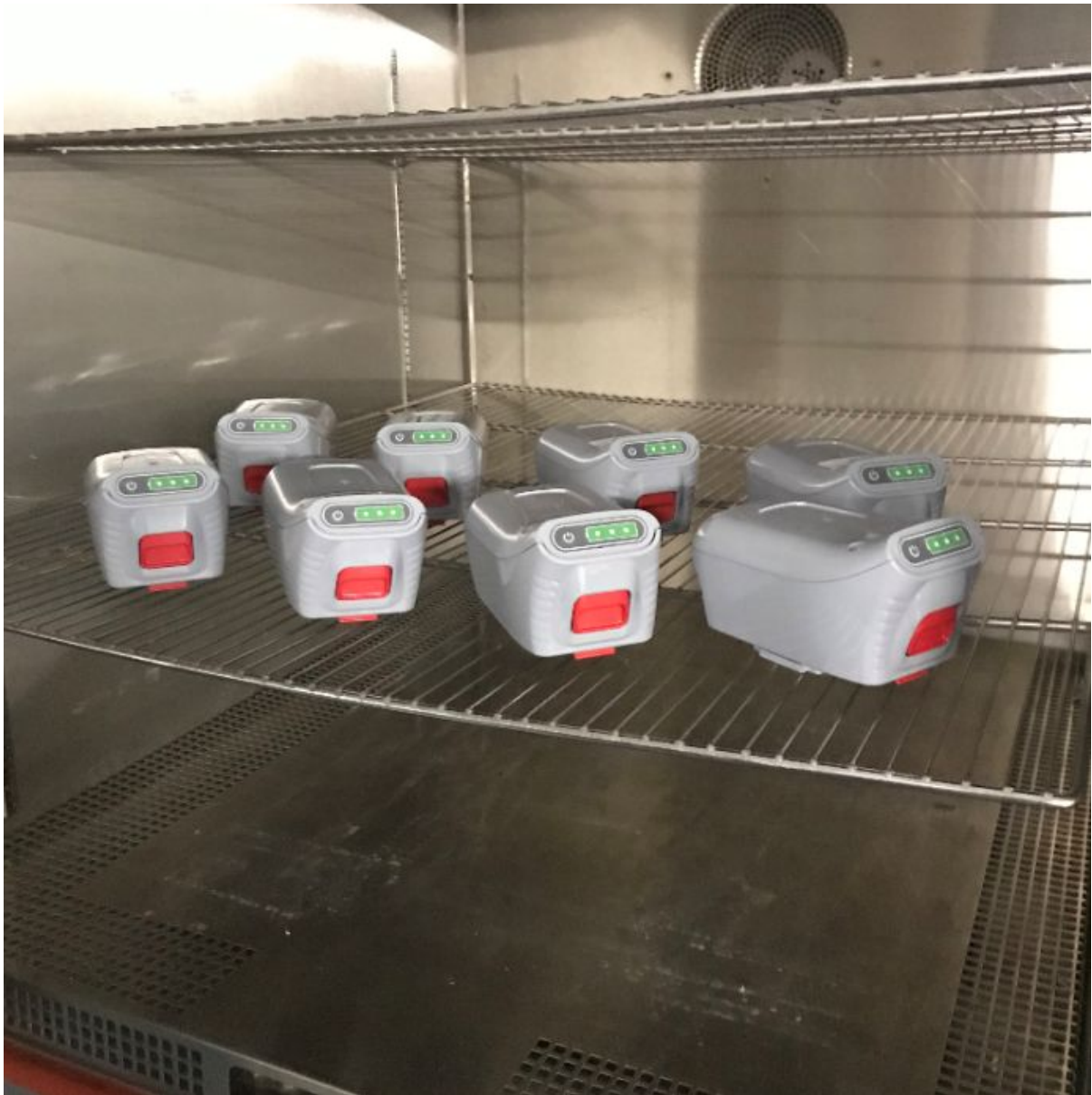
Fig. 2.4 Batteries in T.2 Test setup (Thermal test)
