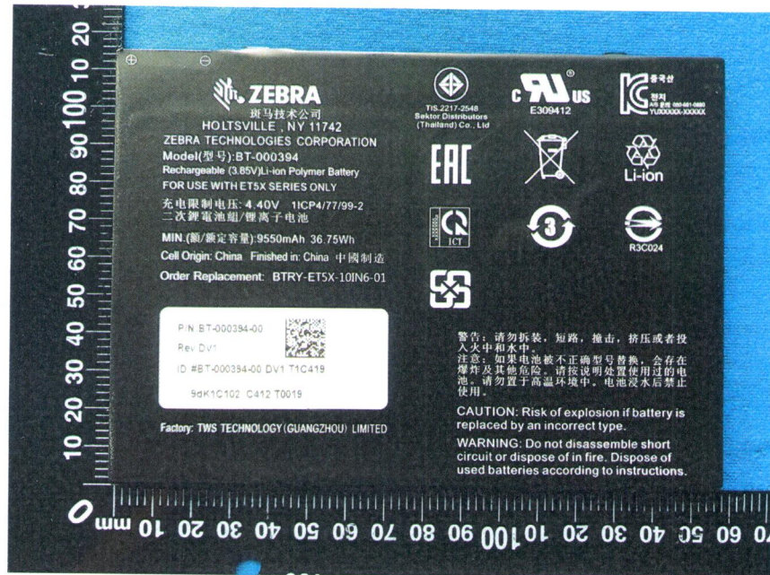
Battery (BT-000394 3.8V 9550mAh 36.75Wh)
