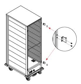
**4.** Replace the M5 screws on the cabinet's right post and tighten fully.
