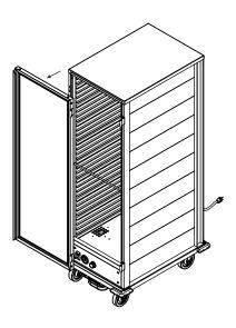
**3.** Use a crosshead screwdriver to remove the M5 screws and remove the hinges on the cabinet's right post.
