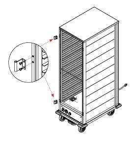
**7.** Install the door to the cabinet's left post and insert the hinge pins.
