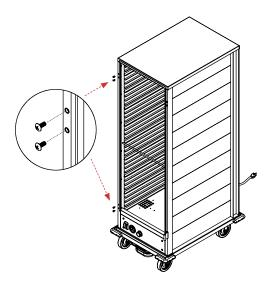
**6.** Install the hinges on the cabinet's left post that were removed from the right post.
