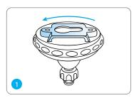
Rotate to separate the base from the bracket.
