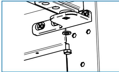
2. Use the wrench to remove the bottom hinge hex screw, then loosen the hinge screws and carefully remove the door.
