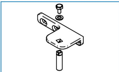
4. Use the wrench to remove the bolt of the top left hinge, then install the bolt into the bottom hinge.
