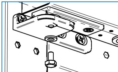
8. Install the hinges on the left side, but do not tighten the screws. Then, install the door and cartridge screw. Tighten all screws.
