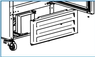
1. Use the Phillips head screwdriver to remove the front panel screws, followed by the front panel.
