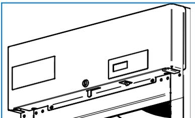
7. Remove the top head screws, then move the hinge cap to the right side. Reinstall the top head screws.
