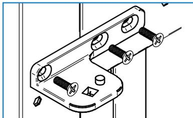
5. Install the bottom right hinge in the top left side of the equipment. Then, install the top right hinge in the bottom left side of the equipment.
