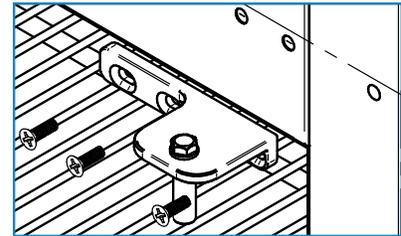
3. Use the screwdriver to remove the bottom and top hinges.
