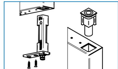
6. Remove the bottom cartridge and bolt housing from the door. Install the cartridge at the top of the door and the bolt housing in the bottom.
