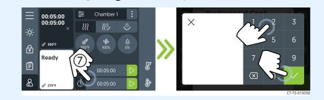
6. **Touch** the cooking temperature **(8)**. **Enter** the cooking temperature using the key pad.
