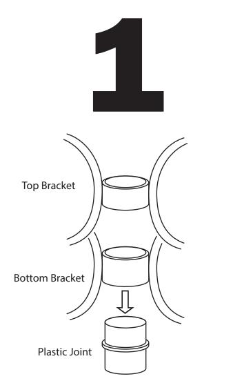
**1. Pull Out the Plastic Joint** From the Bottom Bracket 2. Place the Plastic Joint Between the Top and Bottom Brackets
