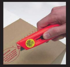
The thumb pushes the button forward & the blade is ready to cut.
