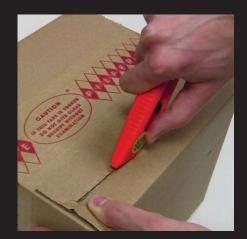
While cutting, the thumb is released. The blade remains engaged & continues to cut, held in place by the box's friction.
