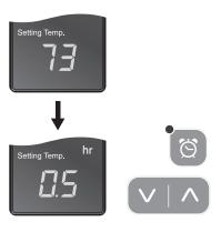
When unit is operating, press the 'Off Timer' button and set the length of time you want by pressing ∧ or ∨.
