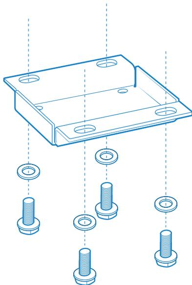
3. Use the screws and washers to fasten the new caster onto the retrofit plate
