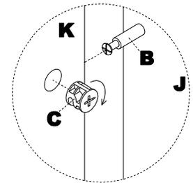
NOTE: The arrow on the face of the Cam (C) should point towards the Cam Post (B) for proper alignment.
