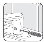
1. With a screwdriver, remove the round tab on the side of the faucet.
