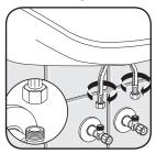
7. Connect braided hose with filter to supply valve. Cold water line has a white label.
