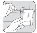
3. Insert anchors into holes and mount LTPS unit to wall with supplied screws.
