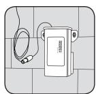
4. Connect spout wire to LTPS connector wire, making sure connectors are oriented correctly.
