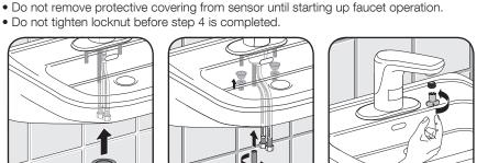
6. Install outlet and tighten with outlet key (supplied).
