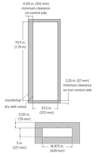
The unit's overall depth is 12.125 inches (308 mm) will sit approximately 11.75 inches (298 mm) below the counter surface depending on counter thickness.
