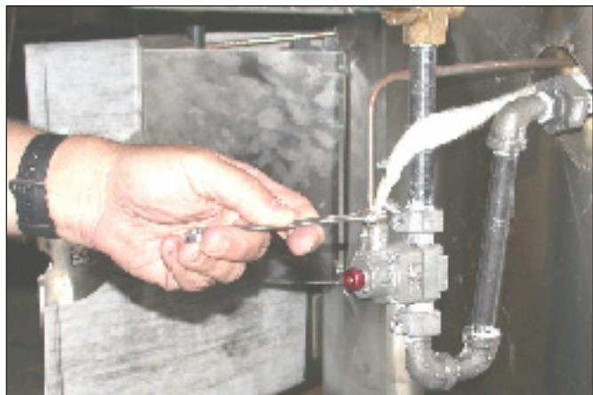
1) Using a 3/8" wrench, remove the brass thermocouple fitting from the safety control
