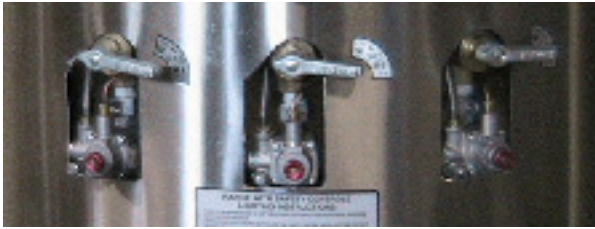
figure A BURNER VALVES IN OFF POSITION— ROTATE COUNTER CLOCKWISE TO TURN ON
