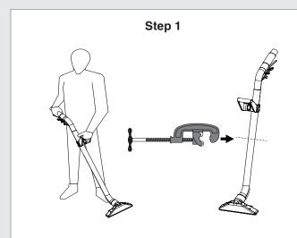
Try the wand for size to decide how much tubing you want to cut off. Proceed to cut the wand tube in half using a tube cutter tool.
