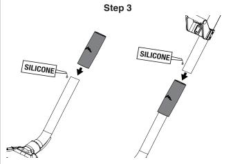
Once you find the right measurements for you, attach the tube coupler. Glue on the included coupler using either a 2-part epoxy (for a more permanent hold) or a silicone adhesive (which can be broken apart at a later date if desired). Use enough adhesive to provide an airtight seal and prevent suction loss.
