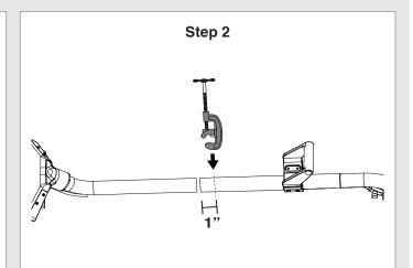
Begin to cut your wand to fit your height. Cut the tubing in 1" increments until you get the right size wand for you. Remember: measure twice, cut once!
