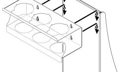
**APPLY DECALS** onto lower face of triple shelf. Clean surface first if needed.
