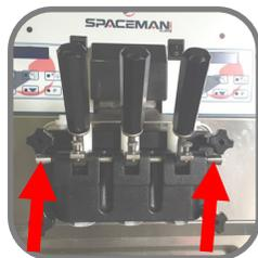
Adjustment screws below draw handles control dispensing speed.
