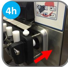
i. Secure door assembly in a cross-pattern using hand-screws (4), with long screws (2) on top
