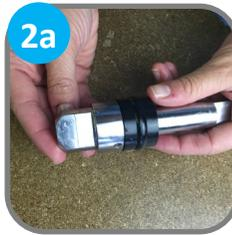
b. Seal gasket open spaces with Spaceman lubricant, extending onto drive shafts and *avoiding the top square parts*
