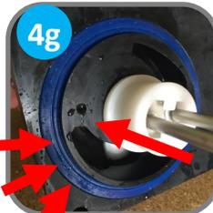
h. Insert dispensing door assembly into cylinders, beater rods first, pushing handles all the way up as you insert
