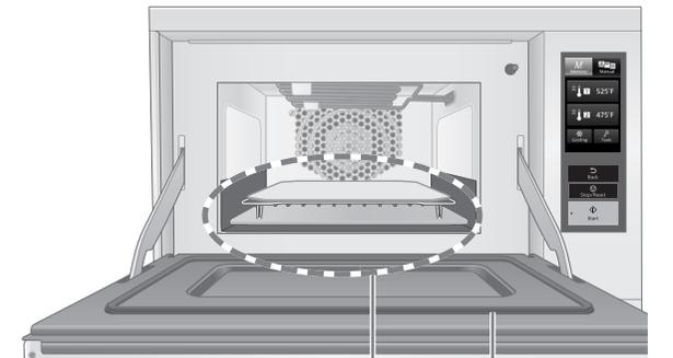
There is a seam in the door seal - this is not damage.
