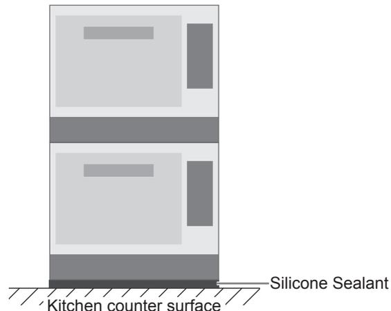
When oven is stacked, its base must be sealed in accordance with NSF Standards as per the following instructions.
