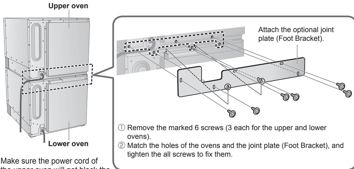
Make sure the power cord of the upper oven will not block the exhaust vent of the lower one.
