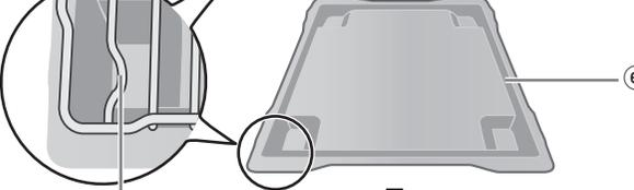
Place the rack so that it is within the tabs of the Ceramic Tray.
