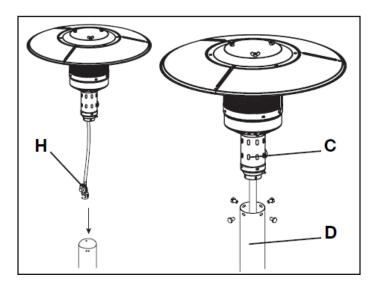
10. Remove the pre-assembled screws from the post support (F) and attach post (D) to the post support (F) using those 4 screws.
