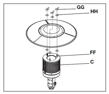
9. Unscrew the four screws that are preassembled on the head assembly (C). Place the head assembly (C) into the top of the post (D) by inserting the regulator (H) into the post (D). Tightly fasten the previously removed screws back into the head assembly (C) through the slots at the top of the post (D).
