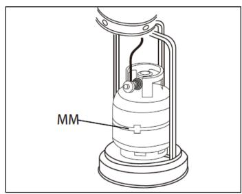
12. Turn the cylinder valve on the tank clockwise to close the propane tank. Attach the regulator (H) to the cylinder valve by turning the regulator coupling nut clockwise. Make sure it is fastened securely and tighten connections by hand only.
