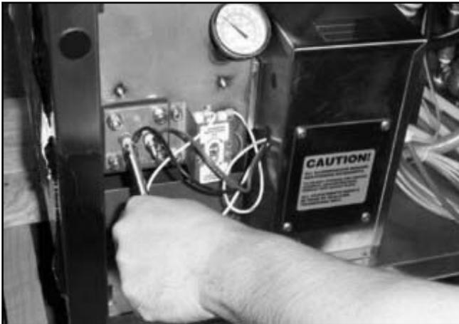
Removing the heater nuts.
