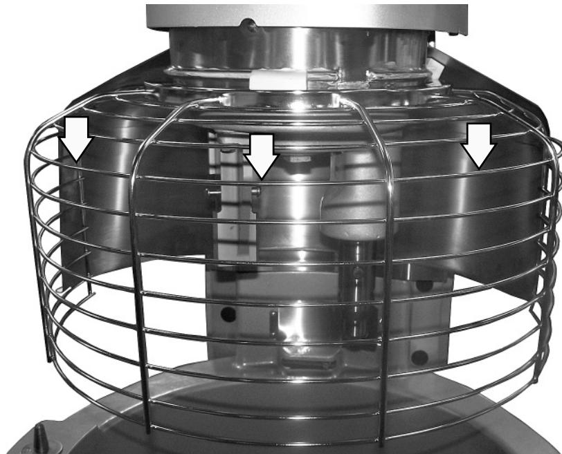
2. Insert the chute between the fifth and sixth wires being sure to engage chute hooks on fourth wire.
