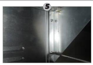
Using screws (#G) to fix the front shelf supports (#F) on the base (#A).
