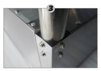
Install legs **(D)** into gussets using screws **(I)**. Make sure the rivet in leg is closer to gusset than to foot end.
