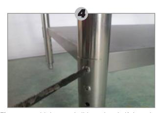
Align under-shelf **(E)** gussets with legs and slide under-shelf down legs to desired position using screws **(J)** to tighten, using the leg plate **(G)** beneath the screws to reinforce the shelf. (DO NOT force or hammer the screws in as damage could occur)
