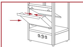
2. Insert panel into unit until side tabs are inside, flexing or rotating door if needed.
