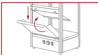
3. Straighten door and lower tabs into cut outs. Flip door up until magnets catch to keep it closed.
