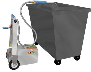
Before stowing the hose/wand <u>rotate the pump in the reverse</u> <u>direction for 6 to 12 rotations</u>. This action will drain the residual waste oil left in the pump and hose back into the **Shortening Shuttle**\* **Pump** thus clearing the pump and minimize dripping of oil from the end of the hose.
