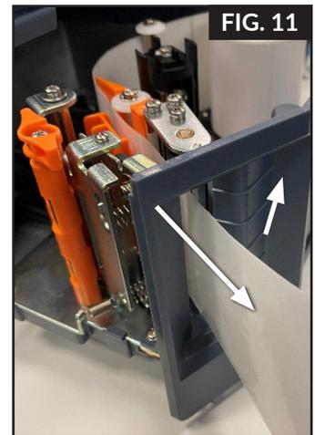
9. Once the label has been pulled through the outside of the printer, take the end of the label roll and run the labels on the left side and out the right side of the final black spool in the middle of the printer. (Fig. 12) Once the label roll has been inserted as shown below, manually spin the spool clockwise to begin wrapping the labels around the spool.
