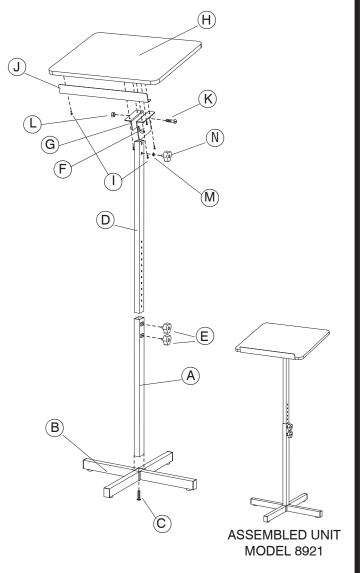
Insert the A Lower Post into the B Base and fasten with the C Bolt (fully threaded) from the underside of the Base.
