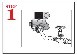
Connect dishmachine to hot water source minimum 120°F required, 140°F temperature recommended.
