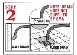
Connect the drain hose to wall or floor drain. The floor drain must have a 1-inch air gap between drain hose and floor drain.
