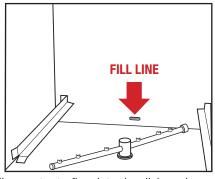
Hold down "FILL" Switch for approximately 10 - 15 seconds to allow water to flow into the dishwasher. Water should reach "FILL LINE" which is located inside at the back of the wash tank. **NOTE:** The 4th cam of timer assembly has to be adjusted to maintain the same water level during the cycle.
