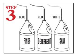
Insert tube stiffener with chemical tubing into each corresponding chemical dispenser.
