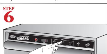
Press and Hold down "SANI", "DETERGENT" and "RINSE" switches to prime chemicals. This step must be repeated each time chemical containers are changed.
